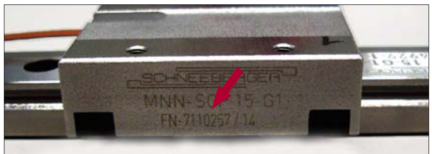
The carriage number is printed on the label of the interface module
