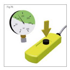
Switch on the hydraulic unit and set the desired pressure using the pressure control valve.
