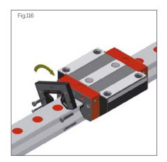
**NOTE**: The lube connections on the front plate are sealed with set screws. During installation of the ZCV/ZBV additional wiper these set screws become covered. When screwing a lube nipple into the additional wiper, the underlying set screws must be removed.
