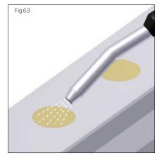
10. Blast loose swarf from the rail surface using compressed air. If necessary, clear remaining swarf using a brass brush. Check that all swarf has been removed.
