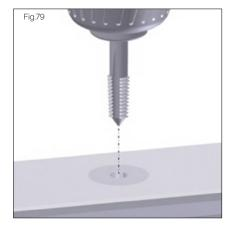
2. Use a thread cutter to cut a thread into the plug. Remove any swarf from the thread.
