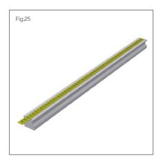
Prior to carriage installation, cover the mounting holes on the upper surface of the guide rail with a suitable adhesive tape. The adhesive tape protects the cross wiper of the carriage from damage by sharp-edged fixing holes.
