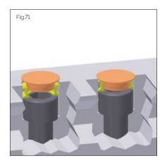
Pressing the plug into the clamping ring causes the latter to expand slightly, applying the ring to the wall of the fixing hole and creating a locking force between the fixing hole and the plug. This functional principle ensures a very firm and secure grip and sealing of the guide rail fixing hole, as well as a flush positioning of the plug in relation to the guide rail surface for the optimal functioning of carriage wipers.
