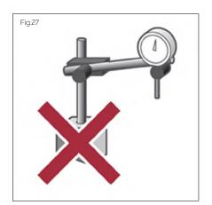
(Fig. 27) Only use non-magnetic aids to transport and align AMS guideways.
