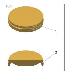
BRS brass plugs have a ring-shaped groove (1). The brass plugs have a recess on their underside (2).
