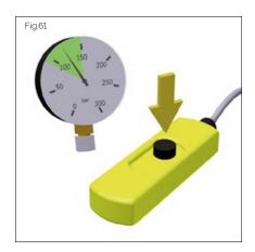
5. Switch on the hydraulic unit and set the desired pressure using the pressure acontrol valve.
