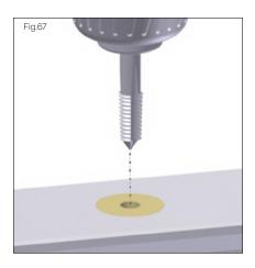
2. Use a thread cutter to cut a thread into the plug. Remove any swarf from the thread.
