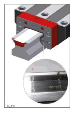
**NOTE**: An absent or interrupted line of lubricant is indicative of an improperly-fitting wiper.
