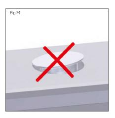
Ensure that the plugs sit plane-parallel to the rail surface in the fixing holes. **NOTE**: The clamping ring has a small recess on the inside of its upper portion that enables the plug to align with it under light pressure.
