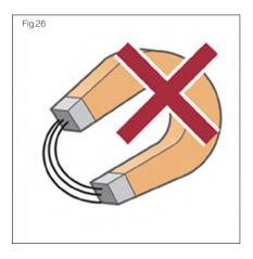
(Fig. 26). Only non-magnetic materials should be used in the direct vicinity of the measuring scale and the read head.
