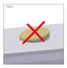
Ensure that the plugs sit parallel to top surface in the fixing holes.
