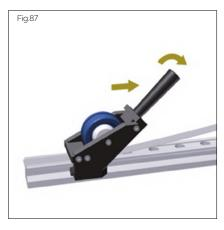
**NOTE**: Do not bend the free strip end at the end of the guide rail. Only move the assembly tool up to the end of the guide rail. Do not move the pressure roller over the end of the guide rail whilst applying pressure.
