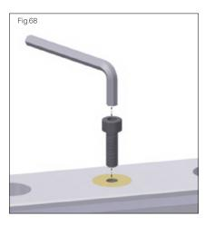
3. Screw the Allen screw into the plug by hand until the tip of the screw comes into contact with the head of the guide rail fastening screw.
