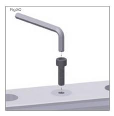
3. Screw the Allen screw into the plug by hand until the tip of the screw comes into contact with the head of the guide rail fastening screw.
