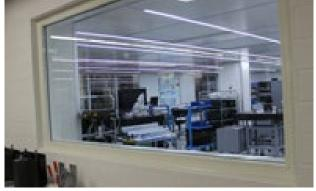
Schneeberger has invested in a modular cleanroom, which meets Class ISO 6 requirements as standard, to be able to supply ultra-clean positioning systems. Even higher standards according to ISO 5 and ISO 4 can be achieved in a separate sub-area.
