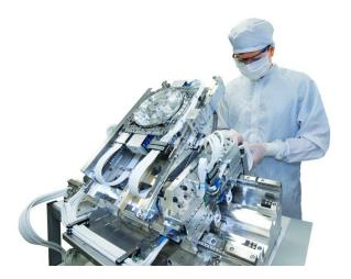
In demand in the semiconductor industry: this high-precision positioning system from Schneeberger is in particular used in wafer production. It's about applying and testing the most delicate structures that form the basis for future semiconductor chips.
