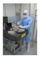
A hood is also part of the standard clothing for specialists working in the ISO 5 and 4 class cleanroom. A filter installed directly over the workstation guarantees optimum air cleanliness.
